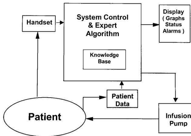
Figure 1. Block diagram of the adaptive patient-controlled analgesia system.
