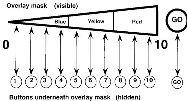
Figure 2. Top view of the patient hand set for the adaptive patient-controlled analgesia system.
